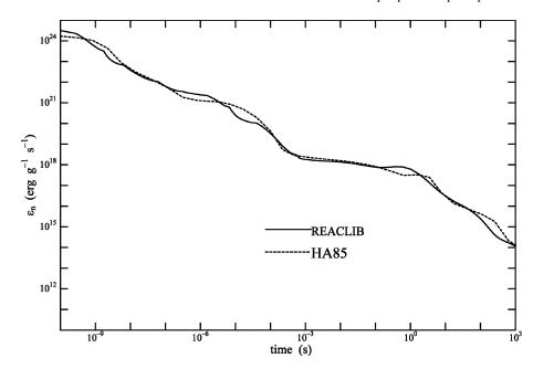
**Fig. 1.** Comparison of the energy generation rate under the constant temperature  $T_9 = 1.5$  and density  $\rho = 10^6$  g cm<sup>-3</sup>. Solid line is the results with the use of new rates (REA-CLIB) and dotted line is those with old rates (HA85).
